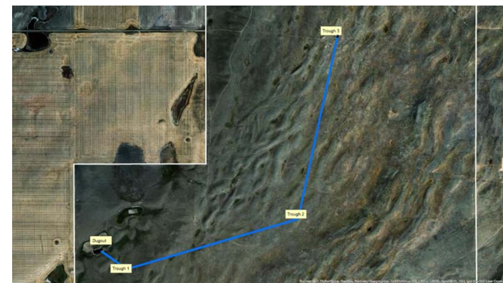
Pasture pipeline from dugout to 3 troughs.
